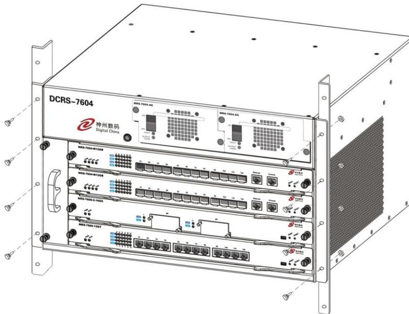
Fig2-3 Rack-mounting DCRS-7604
