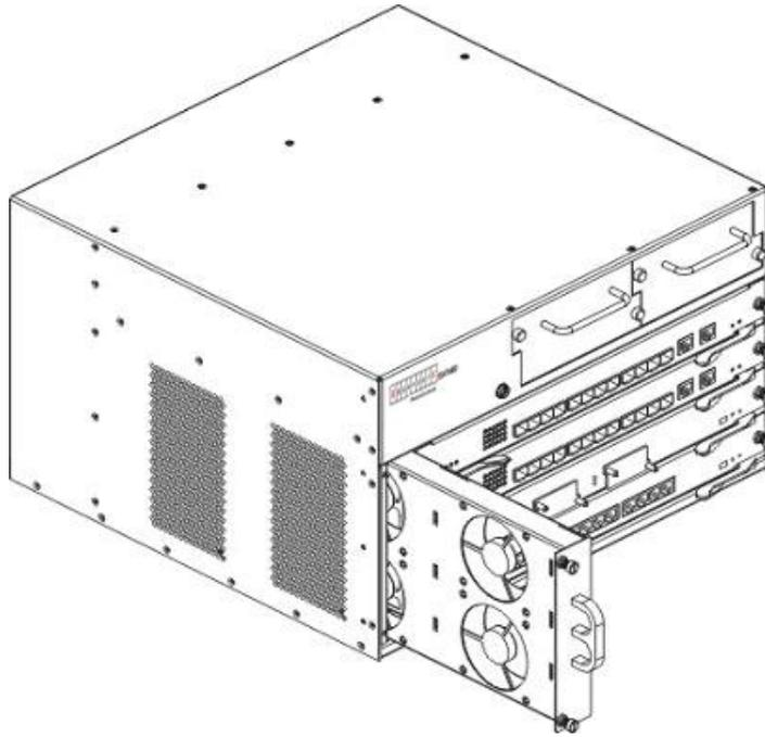
Fig2-7 The installation and removal of DCRS-7604 fan tray
