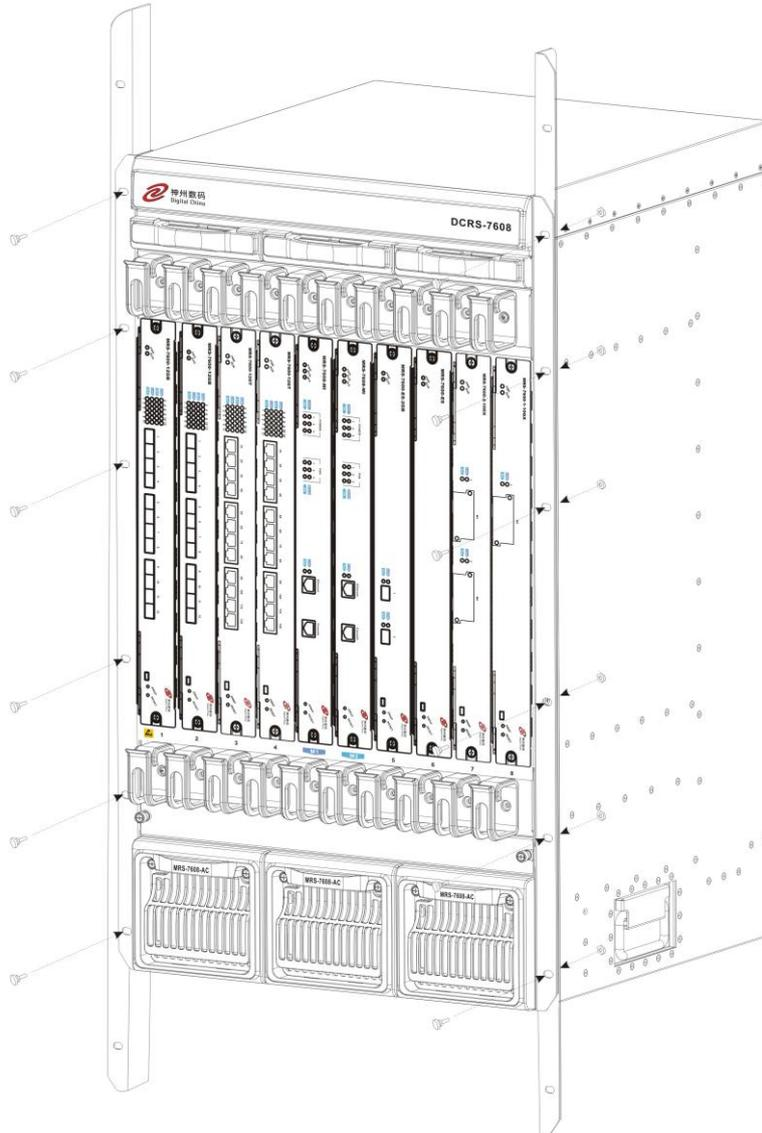
Fig2-4 Rack-mounting DCRS-7608
