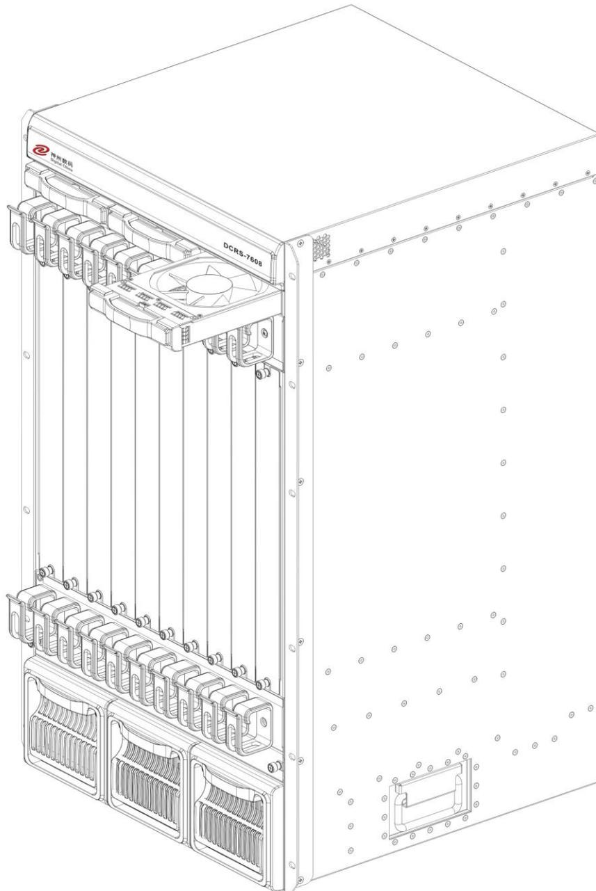
Fig2-8 The installation and removal of DCRS-7608 fan tray
