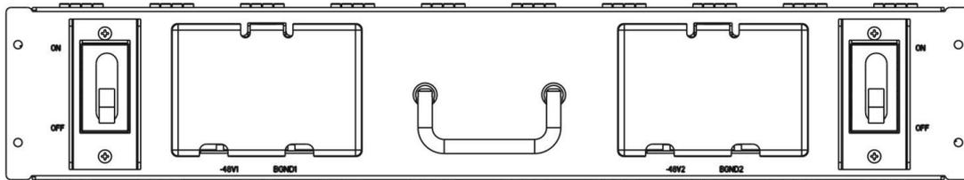
FIG 1-44 DCRS-7608 DC Power Distribution Box
