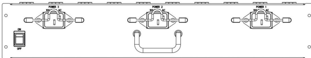
Fig 1-43 DCRS-7608 AC Power Distribution Box
