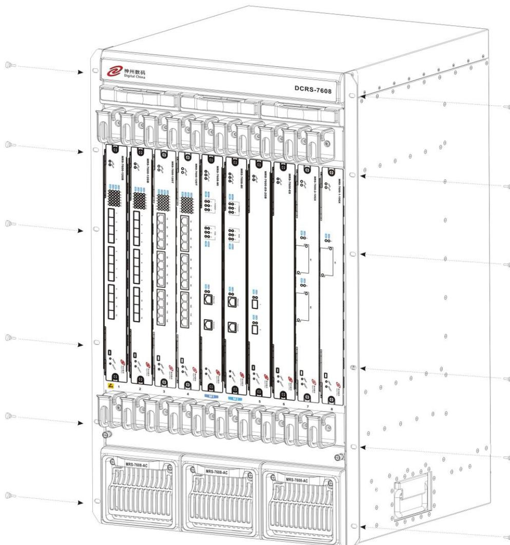
Fig 2-2 Installing DCRS-7608 Switch Hangers
