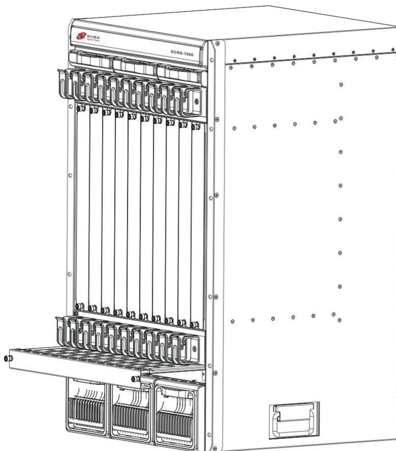
Fig2-6 Installation and removal of the DCRS-7608 dust gauze
