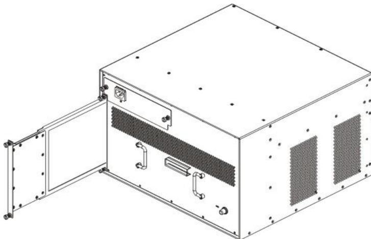
Fig2-5 Installation and removal of the DCRS-7604 dust gauze
