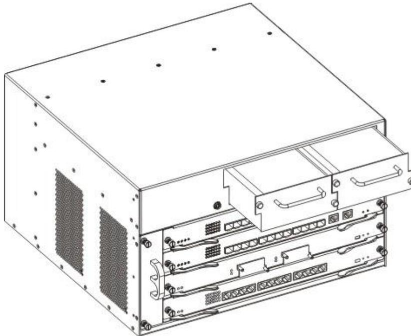
Fig 2-9 the installation and removal of DCRS-7604 power supply modules
