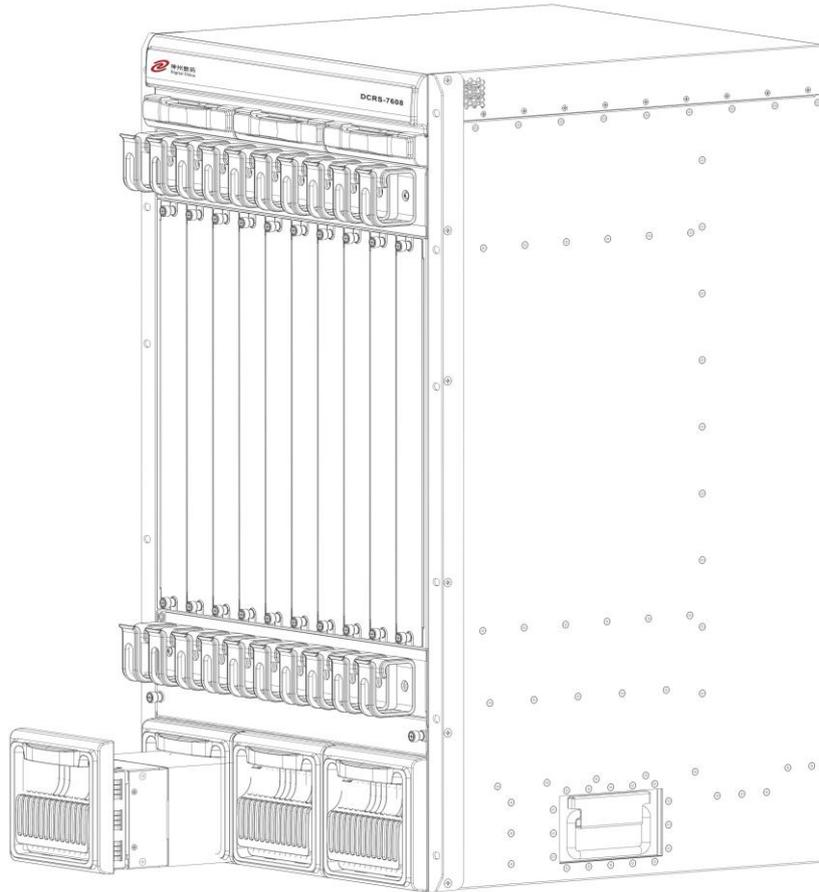
FIG 2-10 The installation and removal of DCRS-7608 power supply modules
