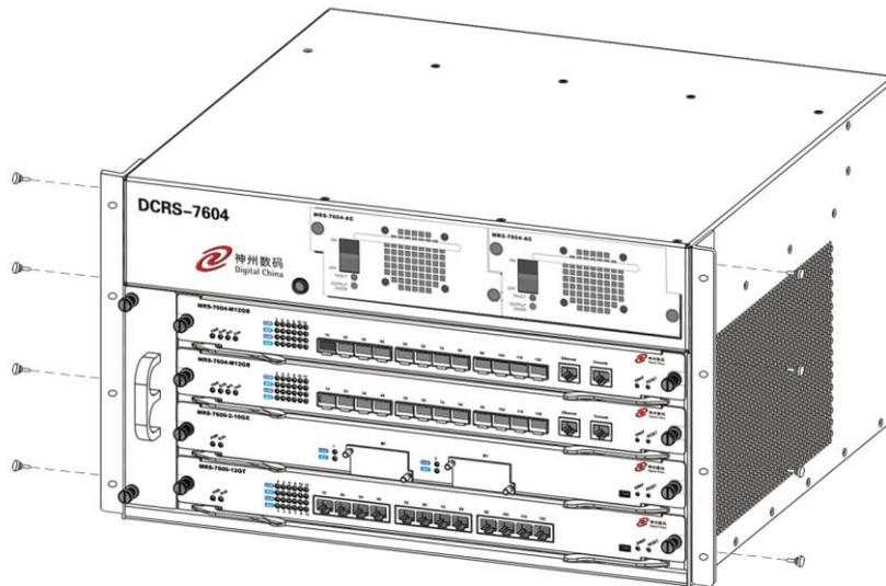
Fig 2-1 Installing DCRS-7604 Switch Hangers
